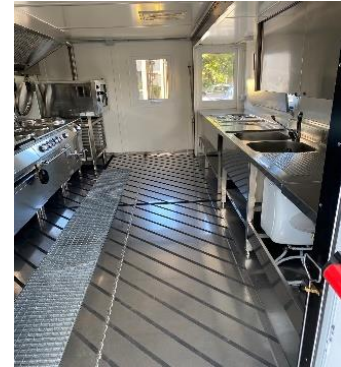
Interior view of the unit from the entrance door and interior view of the volume expanding system, with the distribution area and the sink area "pulled out" from the supporting structure
